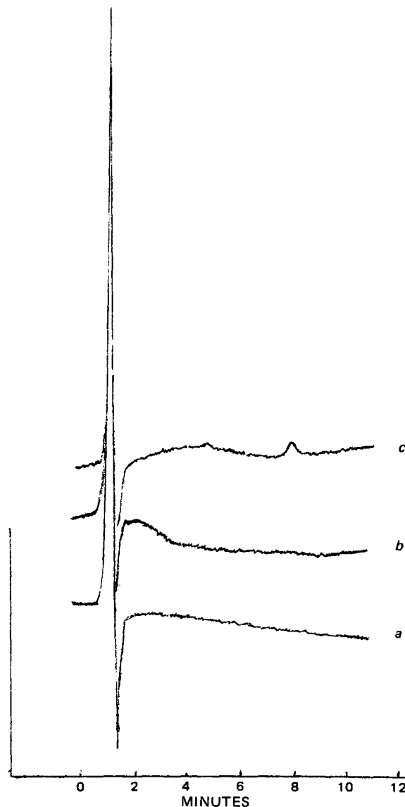
Figure 3—HPLC of pure materials (a) blank, (b) urea, (c) allantoin acid.
